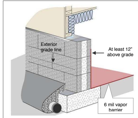
Vapor Barrier Installed in Crawlspace
