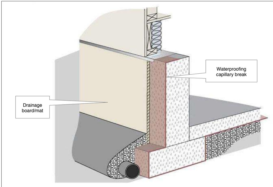
Drainage Plane Applied At Below Grade Wall
