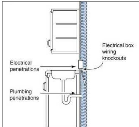
Drywall Penetrations at Building Thermal Envelope
