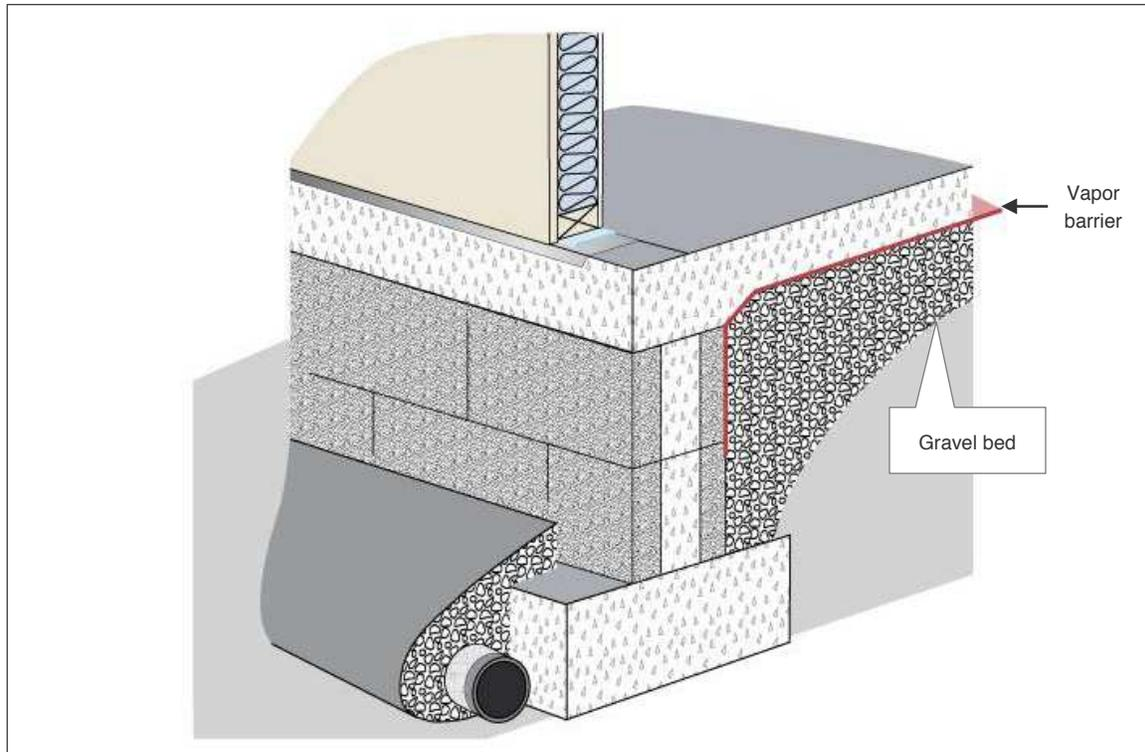
Gravel Bed Beneath Vapor Barrier
