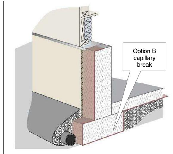
Capillary Break Beneath Footing
